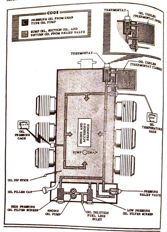
Figure 4. Oil System Schematic
