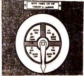
fuel system and allows no fuel to pass beyond the selector valve. The "LEFT TANK" position allows fuel to flow from the left wing tank to the engine.
