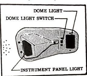
the compass light, is controlled by a rheostat switch (figure 1), labeled "INSTR LIGHTS", located slightly below and to the left of the airspeed indicator. To turn the instrument and compass lights on, rotate the instrument light cheostat switch clockwise until the desired illumination is obtained. To turn the lights off, turn the switch counter-clockwise as far as it will go.
