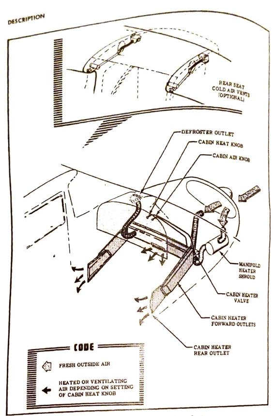
Figure 9. Cabin Air Temperature System
